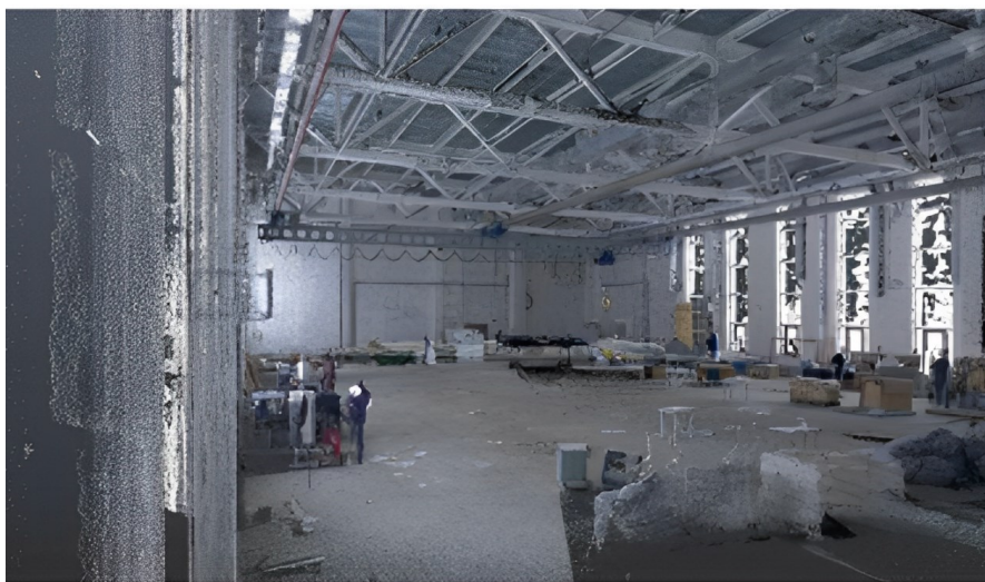
Figure 17- SPbPU Future Factory Point cloud (Badenko et al. , 2019)
