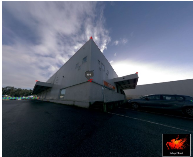
Figure 65 – Marking control points on laser scanner point cloud
