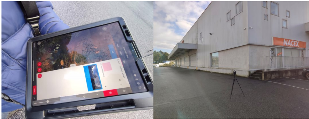
Figure 64 - Laser scanner survey of the warehouse
