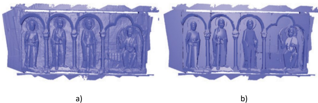
Figure 30 - RANSAC application: a) Point cloud; b) Geometries after RANSAC application (Schnabel, Wahl e Klein, 2007)
