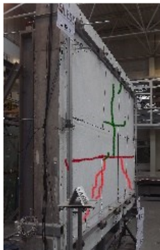
Retrofitted panel (TRM) (max OOP disp. 70mm )
