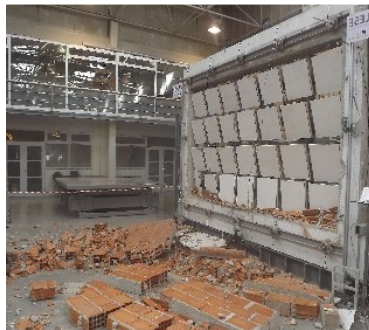
Reference panel (as-built) (max OOP disp. 30mm )
